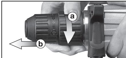
Turn chuck lock (5) as far as it will go (a) in the direction indicated by the arrow, and remove chuck (b).
