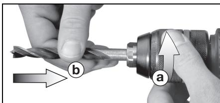
Turn sleeve (4) in the direction of "AUF, OPEN" (a). Insert tool as deeply as possible (b) and turn sleeve in the opposite direction, until the mechanical resistance which can be felt is overcome. **Caution!** The chuck is not yet fully tightened! Keep turning the sleeve (it must "click" when
