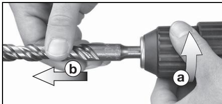
Turn tool lock (3) in direction indicated by arrow (a) and remove tool (b).
