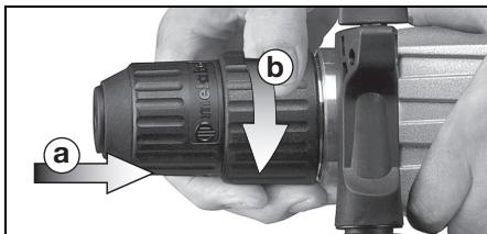
Place chuck onto spindle (6) (a). Turn chuck lock (5) in the direction indicated by the arrow (b) until chuck slides fully onto the spindle. Then release the chuck lock.
